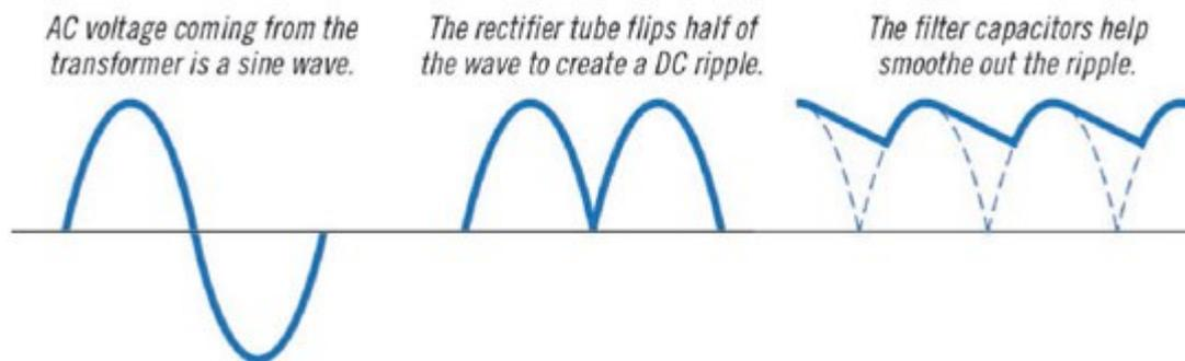
The quality of the charging voltage and charging current is very important. A large ripple is the biggest cause of charger fires. A high current ripple heats up the battery which has an aging effect on the positive electrode. High voltage ripple could harm other equipment that is connected to the battery. CTEK battery chargers produce very clean voltage and current with low ripple.
